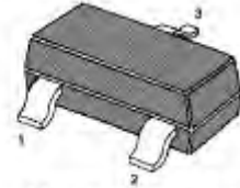
Marking Code: A7 SOT-23 Plastic Package
